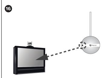
Point the dot (located on the band around the middle of the microphone ball) toward the main display.
