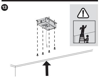
To attach the electronics enclosure, use suitable hardware for your ceiling type. Polycom recommends using four screws and bolts at least 3mm in diameter and at least 25mm in length to mount the electronics enclosure to a solid surface. If the mounting surface is not solid, use an alternative fixing method to ensure that the mounted device can withstand a pull force of 50N without detaching.
