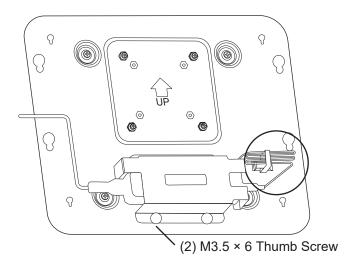
Attach the PC to the plate by sliding the PC holder keyholes onto the four mounting screws.
