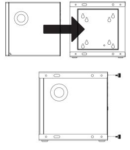
Attach two thumb screws at the bottom of the PSU holder. Wrap the cable wrap around the power cable.
