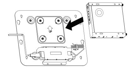
Onnect the cables to the PC. Attach the cable retainers by inserting the two circular ends of each cable retainer into the top of the keyhole slots and sliding them down to lock in place.
