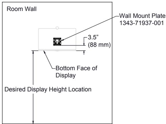
**2** Drill the mounting holes for the wall mount plate as shown using the VESA 100 mm x 100 mm hole pattern. If needed, use the wall plate as a template for drilling the holes.
